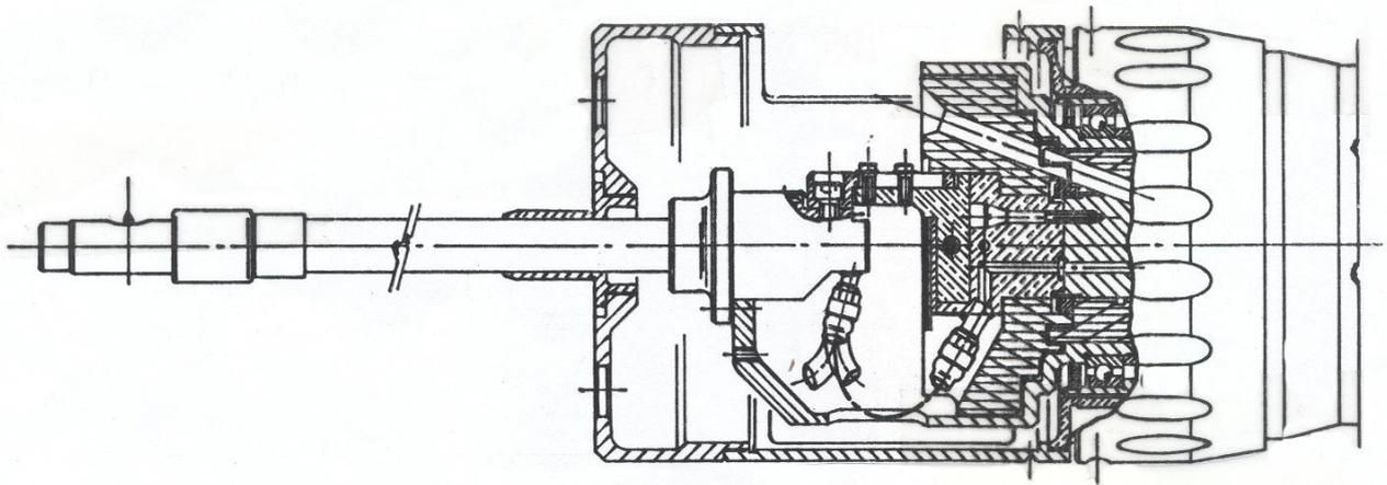
**TORCH FOR INTERNAL TUBE DIAMETER**
